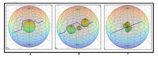
Figure1:Planned path using proposed algorithm a) single static obstacle b) multi static obstacles c) crowded environment
