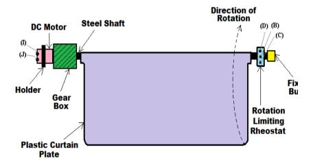
Figure (1): The mechanical unit of the proposed. system.
