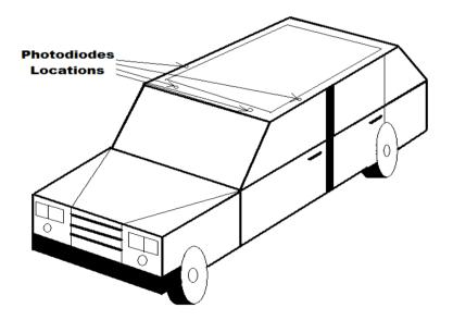
Figure (3): Illustration of four photodiodes location on the car.
